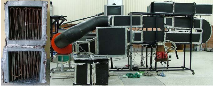
Fig. 4. The prototype: CLOHP/CV air-preheater; and experimental rig.
